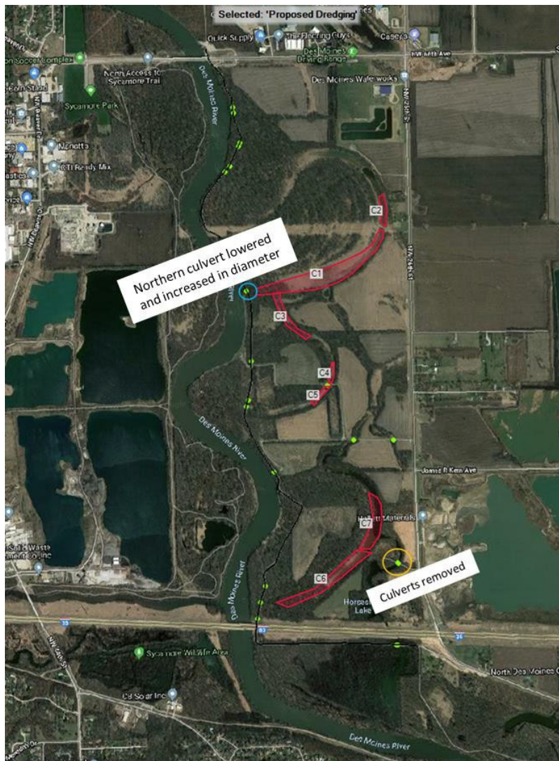
Figure A6: Selected plan – changes to existing condition 2D HEC-RAS model geometry. Red polygons show proposed dredge cuts added to model terrain. Blue circle shows culvert to be lowered and increased in diameter. Orange circle highlights two culverts to be removed.
