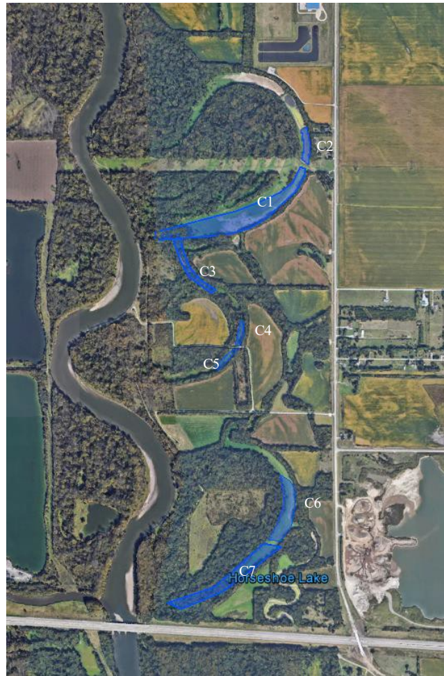
Figure 13: Identified oxbow locations for excavation to create deeper lake-like conditions for purposes of water storage, overwintering fish habitat, and greater habitat diversity.
