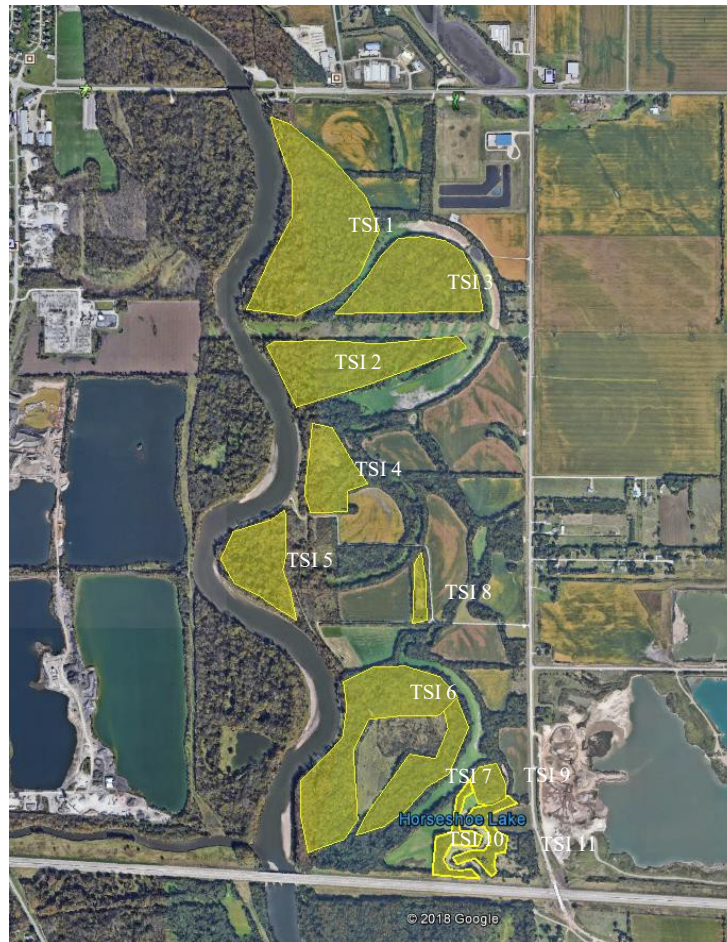
Figure 18: Suitable locations identified as timber stand improvement (TSI 1–11) areas and used as the basis for quantities and cost estimates for restoration.
